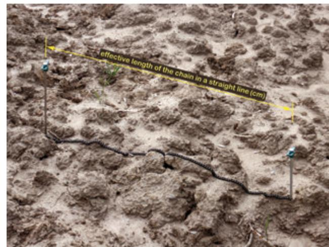
Figure 6. Measurement of the tortuosity index with the chain method. Example of survey of a transect.
