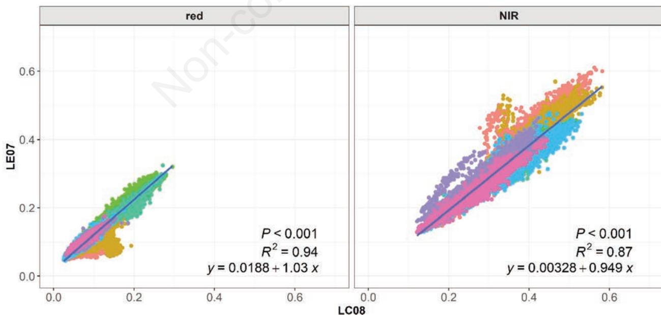
**Figure 2.** Relationships between the spectral reflectance at the red (left) and near-infrared (right) bands detected with LC08 (Landsat-8 operational land imager) and LE07 (Landsat-7 enhanced thematic mapper) and linear regression equation. Different colors represent different groups of sensing dates. NIR, near-infrared.
