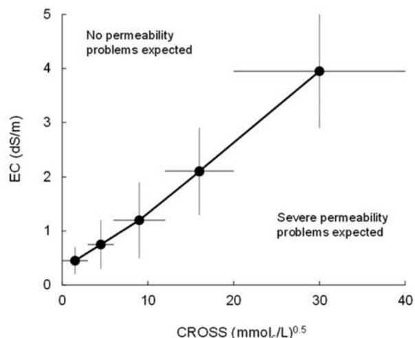
**Figure 4.** Graphic representation of the guidelines for classifying the quality of the irrigation water and assessing soil sodicty hazard using electrical conductivity and cation ratio of structural stability, as proposed by Qadir *et al.* (2021).
