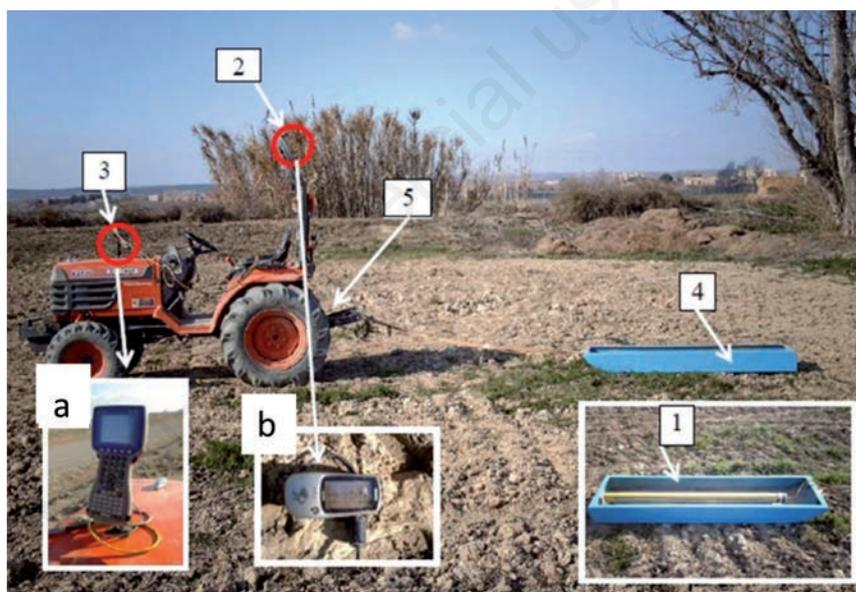
**Figure 3.** Example of a mobile and georeferenced electromagnetic induction sensor with five basic components: 1) electromagnetic sensor [Dualem-1S in (a) and EM38-RT in (b)]; 2) GPS unit; 3) data acquisition system; 4) non-metallic sledge; 5) vehicle. Adapted from Urdanoz *et al.* (2008).
