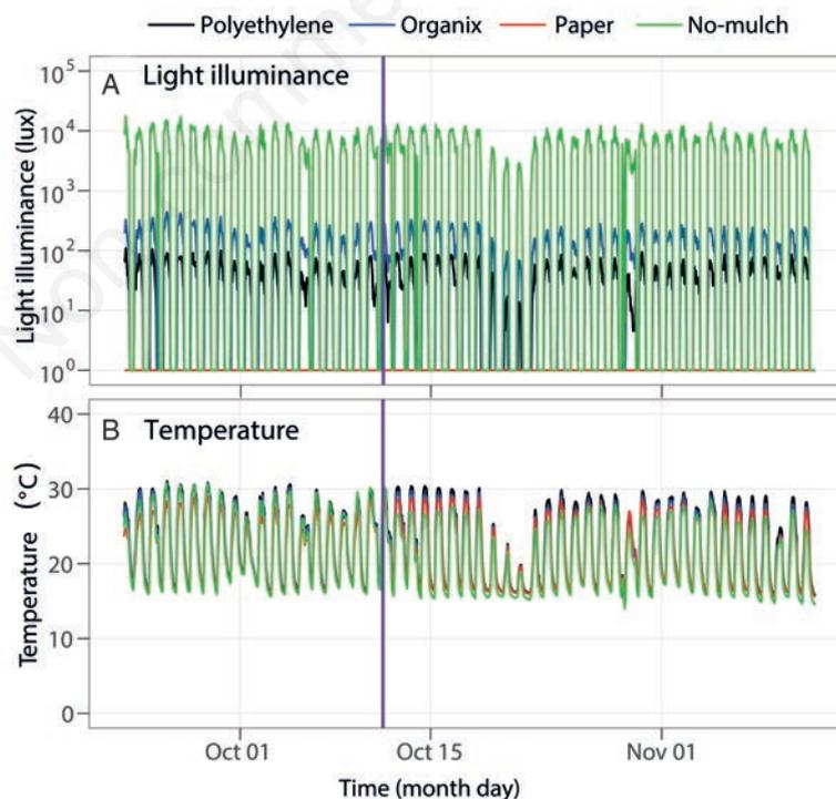
Figure 6. A) Light illuminance and (B) temperature at the soil surface or directly underneath the mulches during the greenhouse study. The vertical purple line indicates when sweet corn was planted. The time tick marks correspond to midnight (00:00 h) for the corresponding day. Assuming the light source was solar radiation, then 122 lux is  $\sim 1 \text{ W m}^{-2}$ . Also, 122 lux will be  $\sim 1 \mu\text{mol m}^{-2} \text{ s}^{-1}$  of photosynthetic photon flux density.
