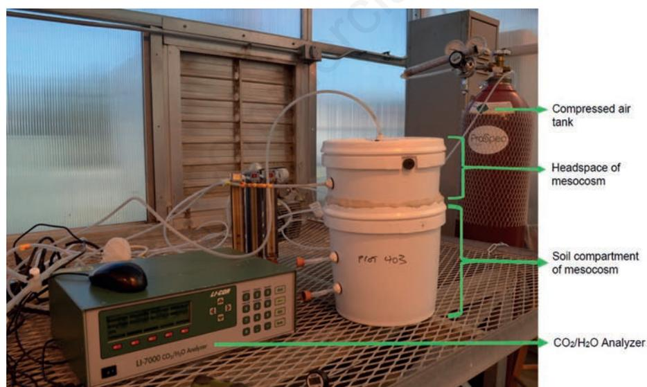
**Figure 1.** Mesocosm setup and simultaneous measurement of CO<sub>2</sub> and H<sub>2</sub>O concentrations over time in the headspace of experimental mesocosm. A schematic of the mesocosm is provided in Figure S1.
