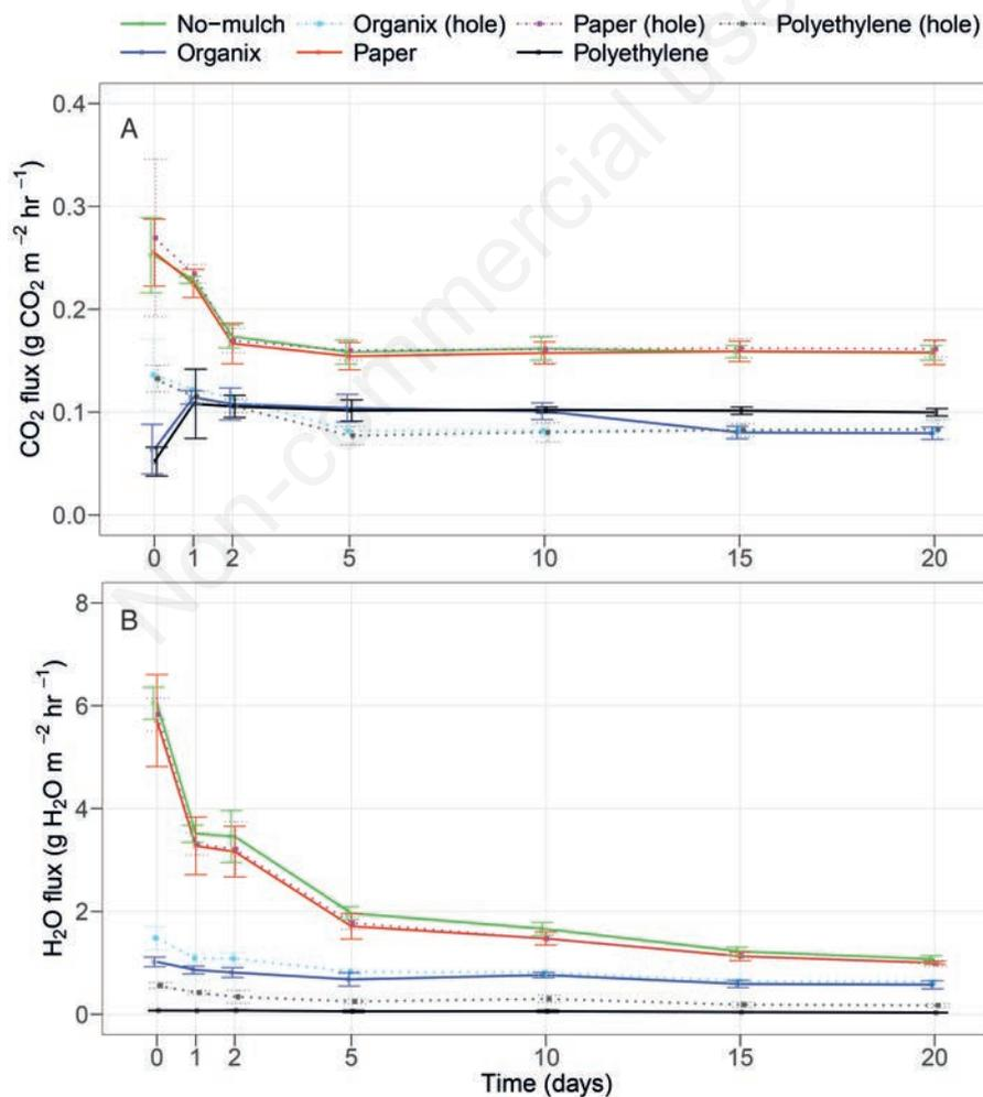
Figure 4. CO<sub>2</sub> and H<sub>2</sub>O diffusive fluxes of the mulch treatments as a function of time in the greenhouse before planting sweet corn. Day 0 refers to the first measurements taken 4–6 h after mulch placement. Error bars indicate the standard deviation of the mean (n=4). Error bars are slightly offset from the x-axis for visibility.
